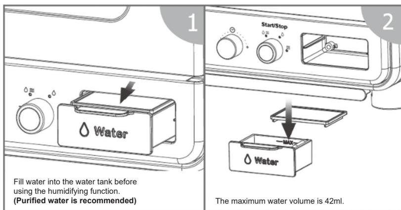
1. Pull out the water tank, remove the lid and fill it up with water to the maximum line before cooking
